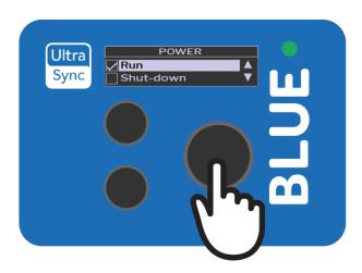
The UltraSync BLUE screen lights up. If it does not light up, the UltraSync BLUE has no power and needs to be charged (see Charging your UltraSync BLUE on page 12).
